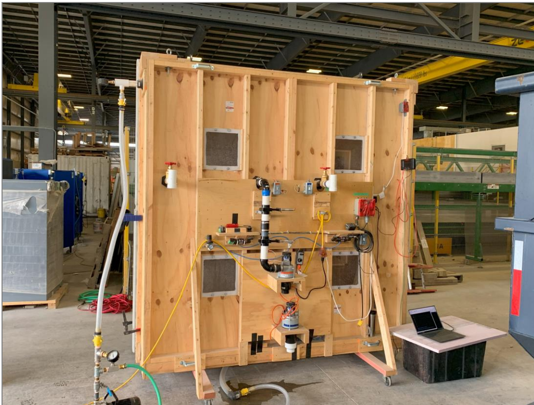
Figure 2.9 - The test chamber during testing is clamped to the test specimen, showing the air pressurization system on the back of the test chamber.
